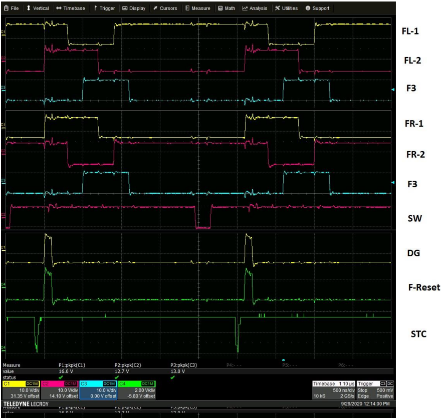
Figure 19 - Serial Right readout waveforms
